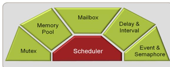
**Fig (4): RTX Structure**
